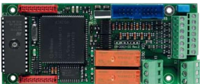
The compact option boards are easily mounted and allow you to combine up to four different options, for example fieldbus communication, motor protection, encoder feedback and crane control.
